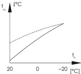
The level needs to be increased and the gradient decreased **if the room temperature drops when it is mild outside.**
