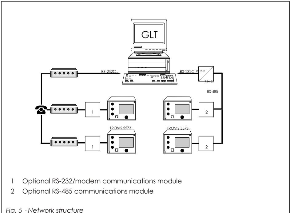
**Note:** The operating software can be updated over the modem or a data cable, provided Modbus is activated by configuring CO6 -> F01 - 1.
